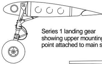
Series 1 landing gear showing upper mounting point attached to main spar
